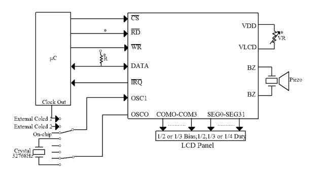
Note: The connection of IRQ and RD pin can sdldcted depending on the requirement of the \(\mu\) C.
